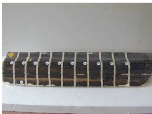
Fig.1. Candoglia marble decayed pillar used in the experimental set up.
