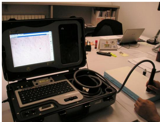
Figure 2. Observation by the optical digital microscope.
