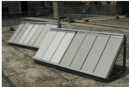
Figure 1. The exposure of the samples on the flat cover of a building of the Politecnico of Milan.
