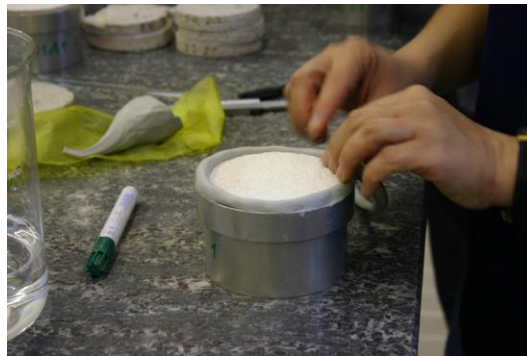
Figure 4. A capsule for the test of permeability to water vapour.
