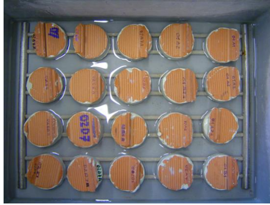
Figure 4. The cylindrical test pieces immersed in water for permeability of liquid water test.
